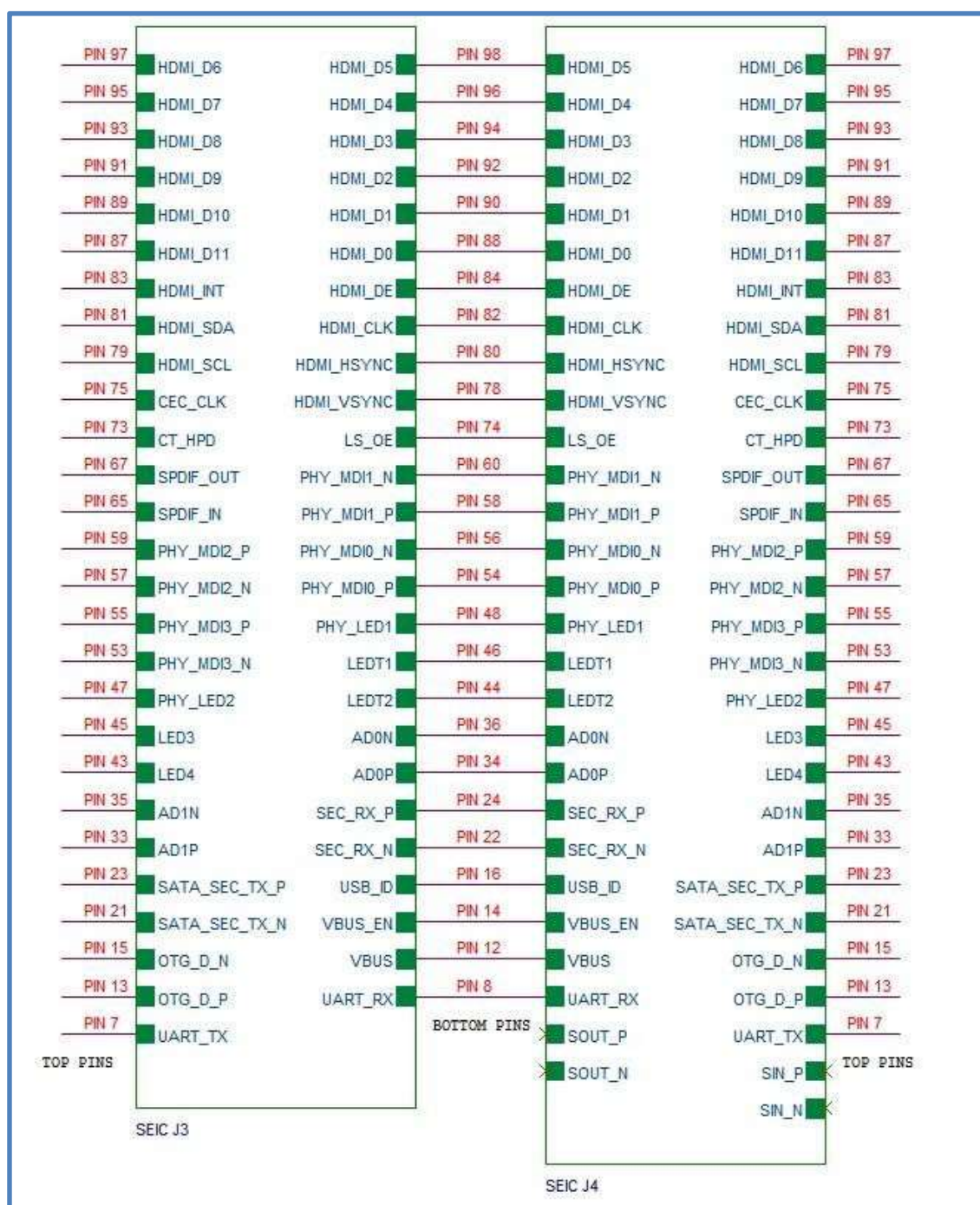
Figure 15 - SEIC Connector Pinout
