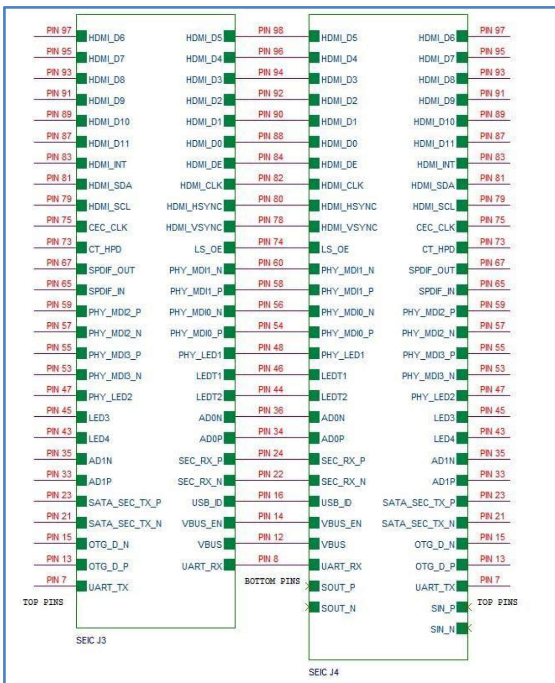
Figure 15: SEIC Connector Pinout
