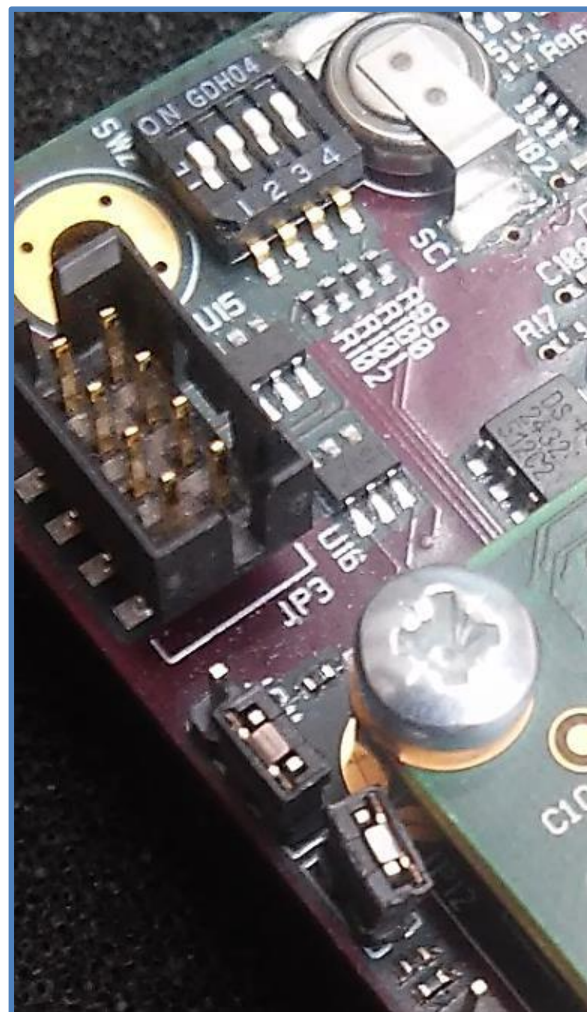
Figure 11: JP12 sets the host mode, SW2 selects port 0 as upstream port
